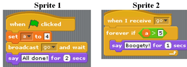
Figure (2.6) Code demonstrating the behavior of the blocking broadcast command.
