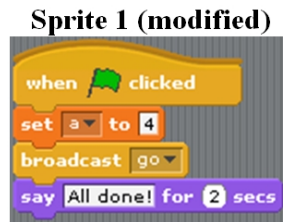
Figure (2.7) Code demonstrating the behavior of the non-blocking broadcast command.
