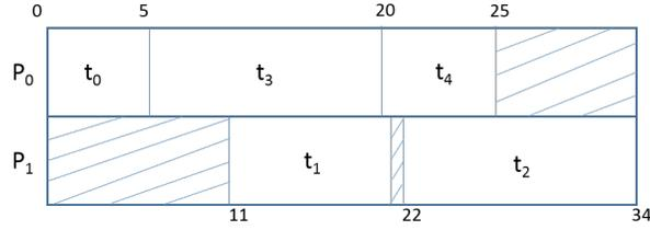
Figure 11.4: A Gantt chart representing a schedule for the task graph shown in Figure 11.3 on a machine with two processors  $P_0$  and  $P_1$ . The shaded area represents the waiting time for each processor based on the task communication delays, assuming the tasks are initially located at processor  $P_1$ .
