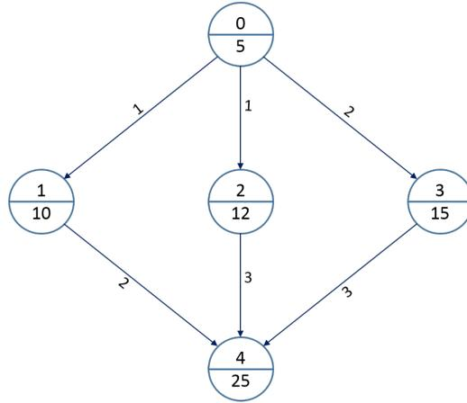
Figure 11.3: A task graph with five tasks represented as nodes showing task numbers and task execution times (for example, milliseconds), and directed edges, indicating the order of execution of tasks, labeled with communication costs.
