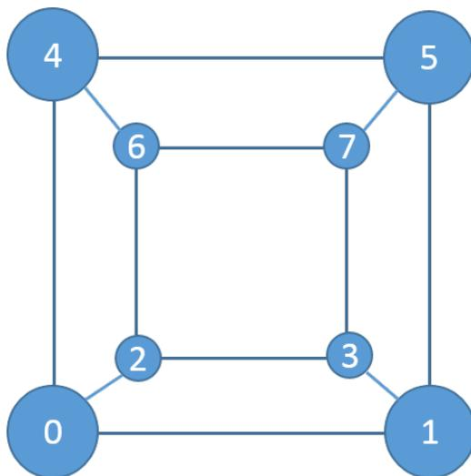
Figure 11.2: An example of a target machine with eight processors ( $m = 8$ ) forming a three dimensional hypercube network. The nodes are labeled with integers indicating the processor numbers.
